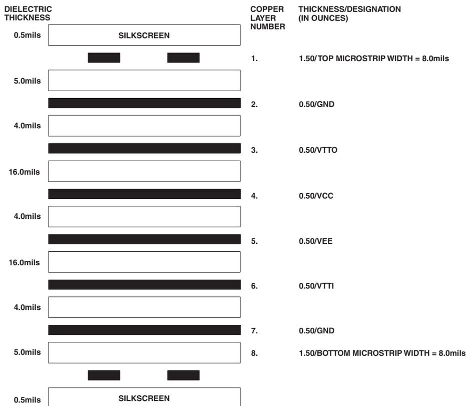
Figure 11. Evaluation Board Stack-Up
