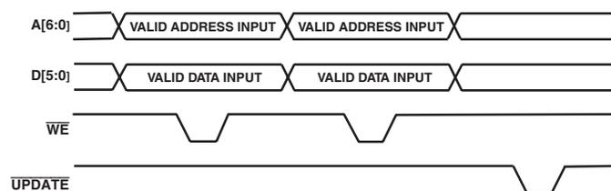
Figure 6. Programming Waveforms
