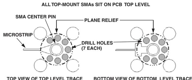
Figure 10. Top-Mount SMA PCB Layout, Two Views
