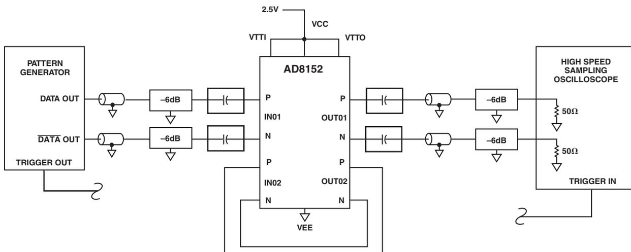
VCC = VTTI = VTTO = 2.5V, VEE = 0V, I<sub>OUT SET</sub> = 16mA
