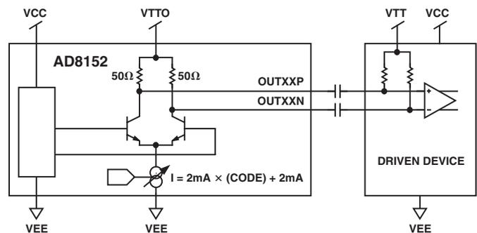
Figure 8. AC-Coupling Output Signal from AD8152
