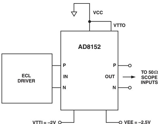
Figure 15. Evaluation Board ECL Driver Test Setup
