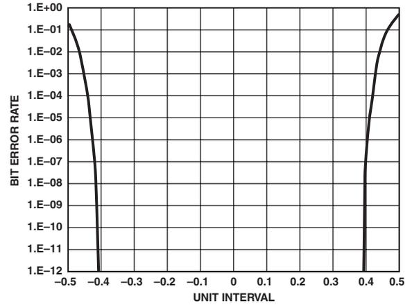
TPC 10. Bit Error Rate vs. Unit Interval
