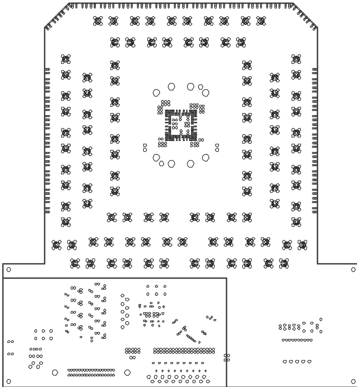
Figure 20. Evaluation Board VCC Layer, View from Top
