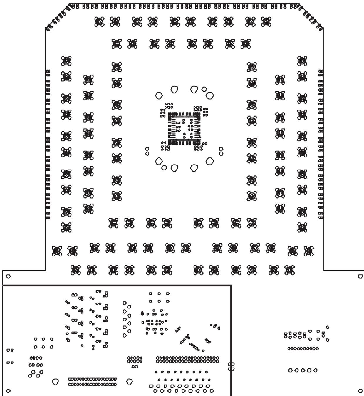
Figure 22. Evaluation Board VTTI Layer, View from Top
