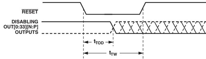
Figure 5. Asynchronous Reset
