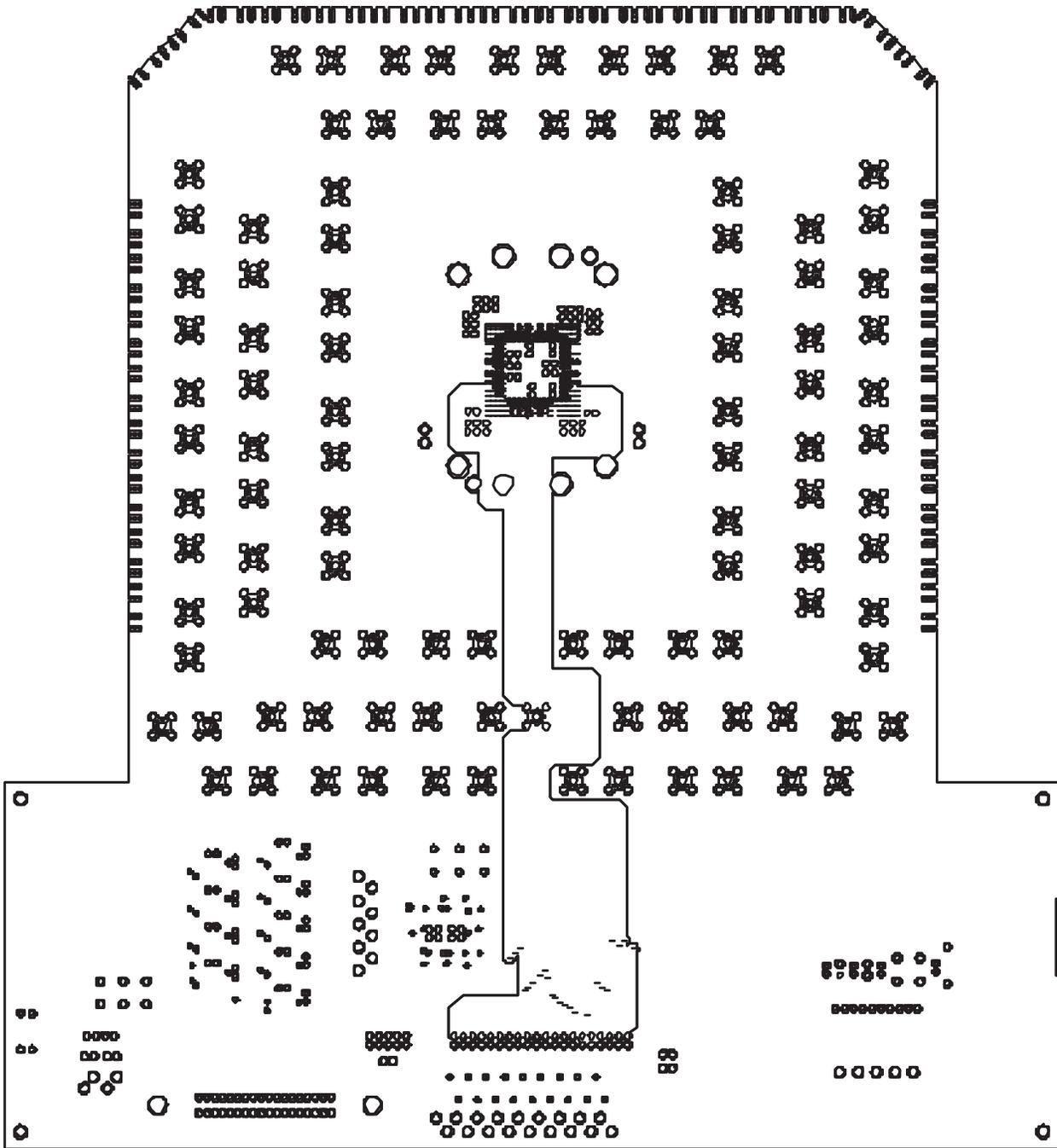
Figure 23. Evaluation Board VTT0 Layer, View from Top
