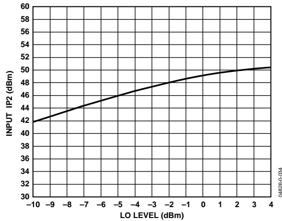
Figure 14. Input IP2 vs. LO Power, F_{RF} = 890 MHz, F_{LO} = 1090 MHz (RF Tone Spacing = 50 MHz)
