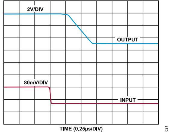
Figure 26. Differential Overload Recovery, Falling,  $V_S = 5\text{ V}$
