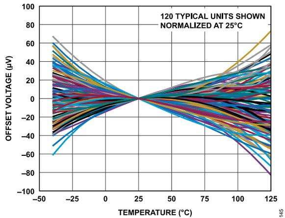
Figure 6. Offset Voltage vs. Temperature, Normalized at 25°C
