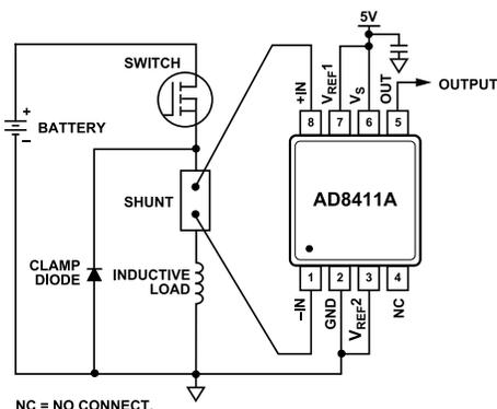
Figure 61. High-Side Switch
