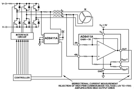
Figure 1. AD8411A in BLDC Motor Control Application
