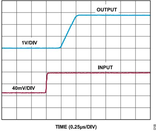
Figure 23. Differential Overload Recovery, Rising,  $V_S = 2.9\text{ V}$
