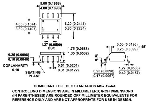
Figure 66. 8-Lead Standard Small Outline Package [SOIC\_N] Narrow Body (R-8)
