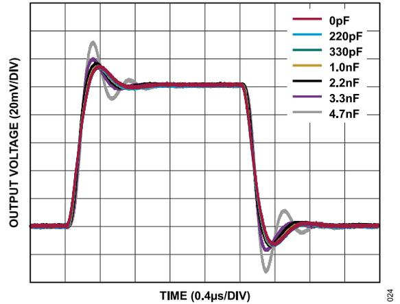
Figure 27. Small Signal Response for Various Capacitive Loads
