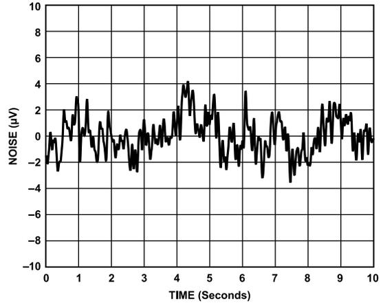
Figure 38. 0.1 Hz to 10 Hz Noise, RTI
