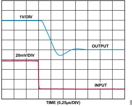
Figure 29. Large Signal Response, Falling,  $V_S = 5\text{ V}$
