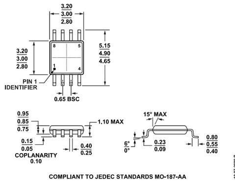
Figure 67. 8-Lead Mini Small Outline Package [MSOP] Narrow Body (RM-8)
