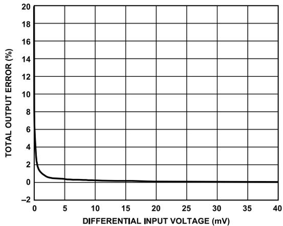
Figure 13. Total Output Error vs. Differential Input Voltage
