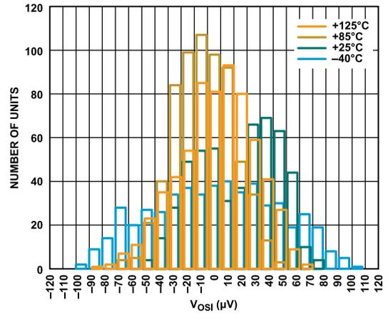
Figure 44. Offset Voltage ( $V_{OS}$ ) Distribution, RTI
