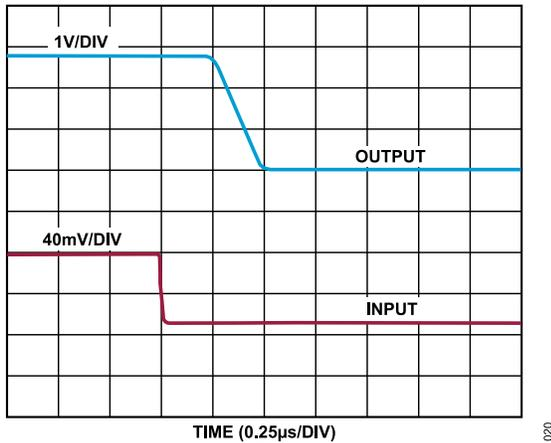
Figure 25. Differential Overload Recovery, Falling,  $V_S = 2.9\text{ V}$
