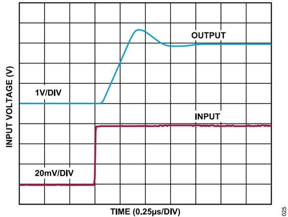
Figure 28. Large Signal Response, Rising,  $V_S = 5\text{ V}$
