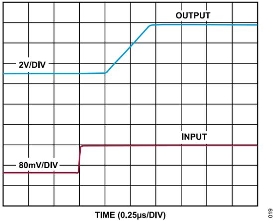
Figure 24. Differential Overload Recovery, Rising,  $V_S = 5\text{ V}$
