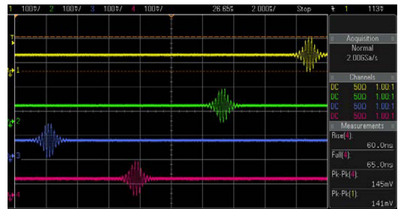
Figure 59. Programming Example 5: Four Pulsed DDS-Generated Sine Waves Amplitude modulated by an SRAM Vector with Different Start Delay
