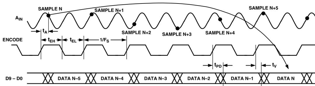
Figure 1. Timing Diagram
