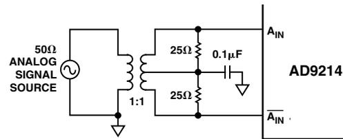
Figure 8. Single-Ended-to-Differential Conversion Using a Transformer
