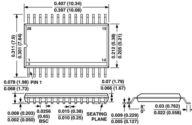
CONTROLLING DIMENSIONS ARE IN MILLIMETERS; INCH DIMENSIONS ARE ROUNDED-OFF MILLIMETER EQUIVALENTS FOR REFERENCE ONLY AND ARE NOT APPROPRIATE FOR USE IN DESIGN
