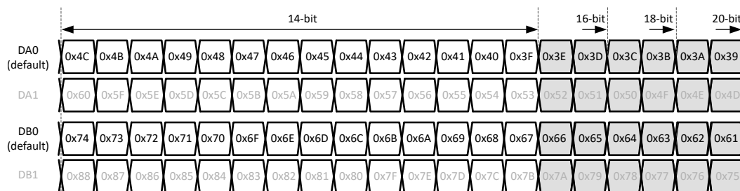
Figure 8-38. 1-wire output bit mapping
