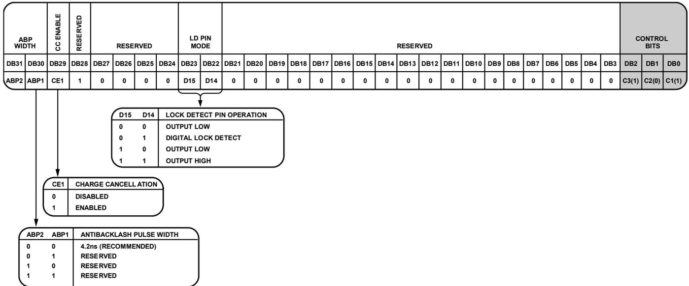
\*MUXOUT IN REGISTER 2 MUST ALSO BE SET TO DIGITAL LOCK DETECT FOR THE LOCK DETECT PIN TO OPERATE CORRECTLY.
