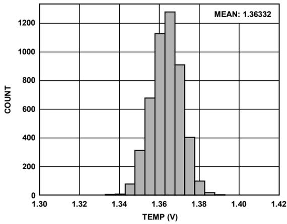
Figure 40. Distribution of TEMP Pin Voltage for 4000 Devices
