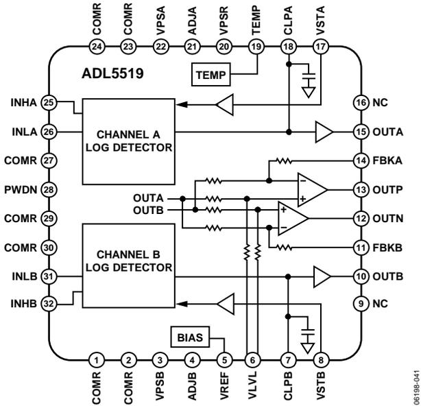
Figure 50. Block Diagram
