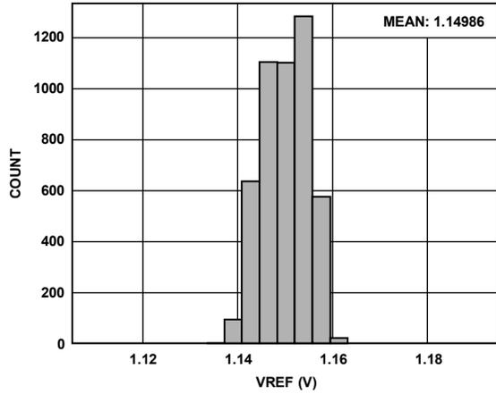
Figure 39. Distribution of VREF Pin Voltage for 4000 Devices
