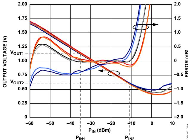
Figure 60. Transfer Function at 2.2 GHz with Calibration Points
