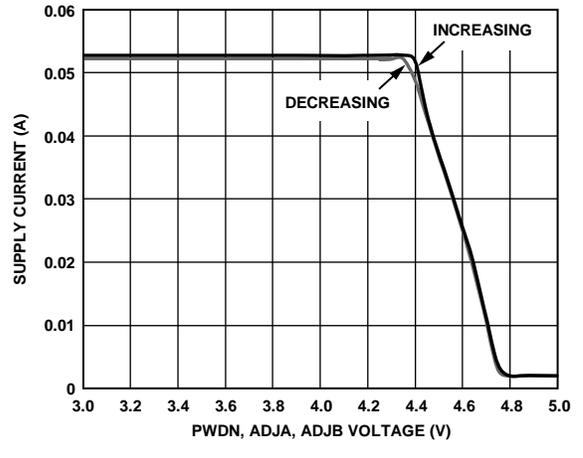
Figure 49. Supply Current vs.  $V_{PWDN}$ ,  $V_{ADJA}$ ,  $V_{ADJB}$
