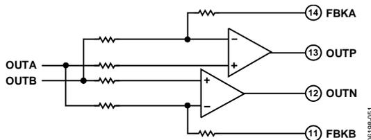
Figure 58. Op Amp Connections (All Resistors Are 1 kΩ ± 20%)
