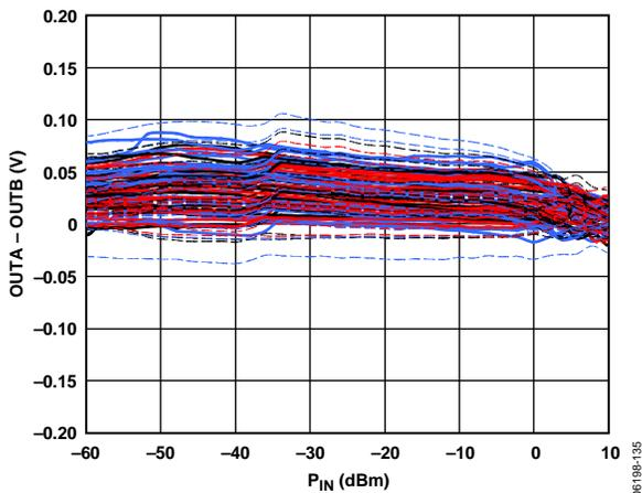
Figure 35. Distribution of [OUTA - OUTB] Voltage Difference over Temperature for 45 Devices from a Nominal Lot, Frequency = 8 GHz, ADJA, ADJB = 0.72 V, 0.82 V, Sine Wave, Single-Ended Drive
