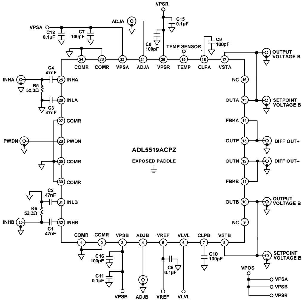
Figure 53. Basic Connections for Operation in Measurement Mode
