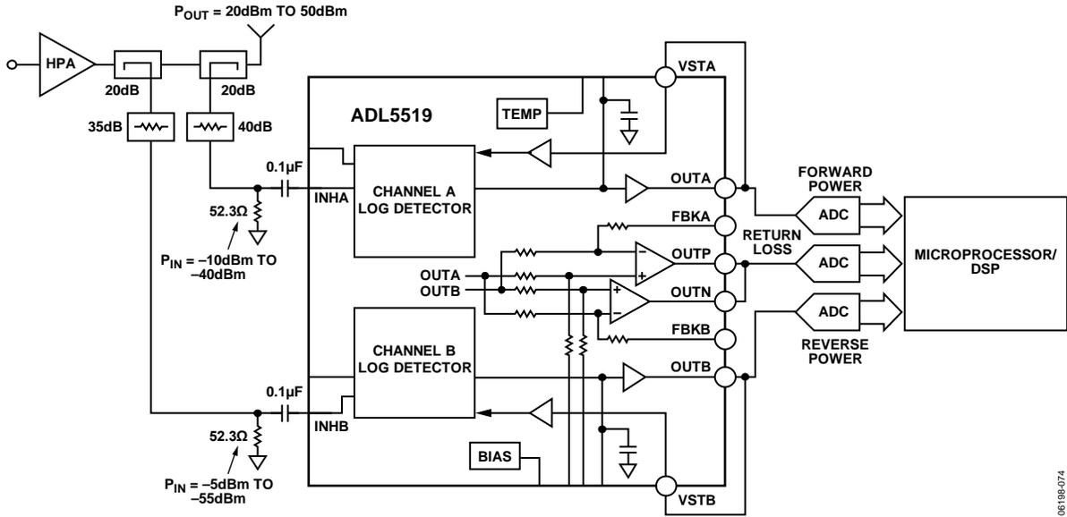
Figure 71. ADL5519 Configuration for Measuring Reflection Coefficients
