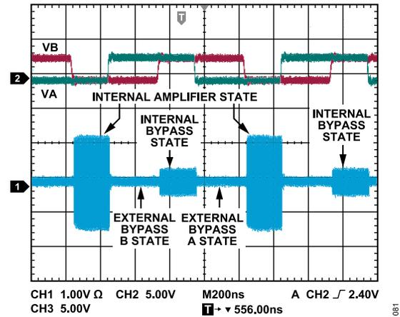
Figure 82. Time Domain Response of RFOUT to Switching of VA and VB Voltages with a Continuous 2.5 dBm RF Input
