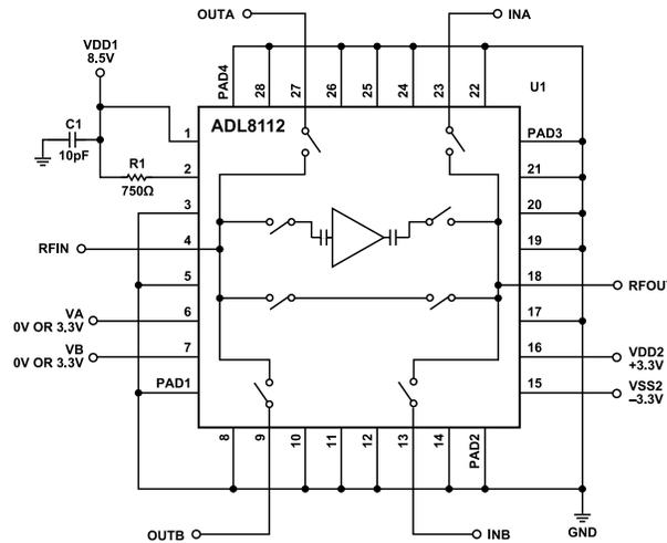
Figure 83. Basic Connections and Evaluation Board Schematic
