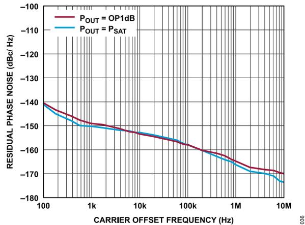
Figure 41. Phase Noise at 5 GHz
