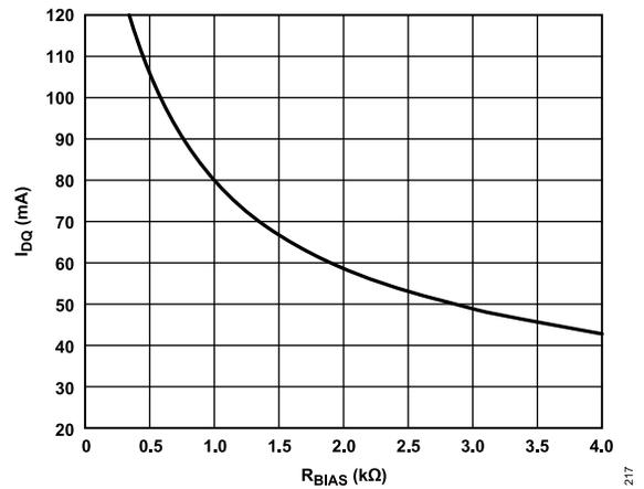
Figure 17.  $I_{DQ}$  vs.  $R_{BIAS}$ ,  $V_{DD} = 8.5$  V
