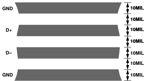
Figure 19. Arrangement of Signal Tracks
