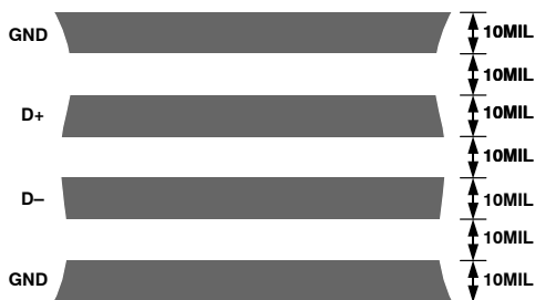
Figure 34. Arrangement of Signal Tracks
