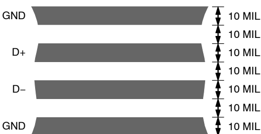
Figure 19. Arrangement of Signal Tracks
