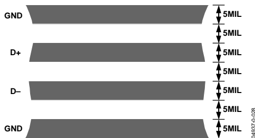
Figure 29. Arrangement of Signal Tracks
