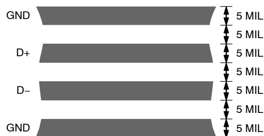
Figure 28. Arrangement of Signal Tracks
