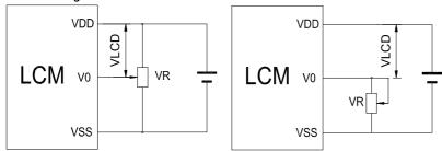
$V_{DD\sim}V_0$ : LCD Driving voltage VR:  $10k\sim20k$
