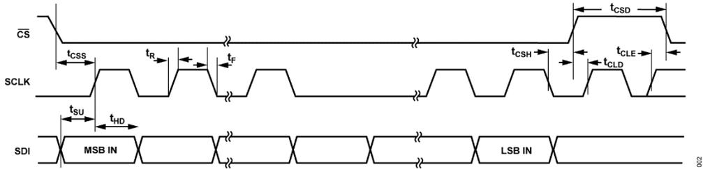
Figure 2. SPI Controller Request Timing Diagram
