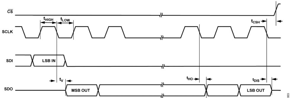
Figure 3. SPI Timing Diagram for Subordinate Response
