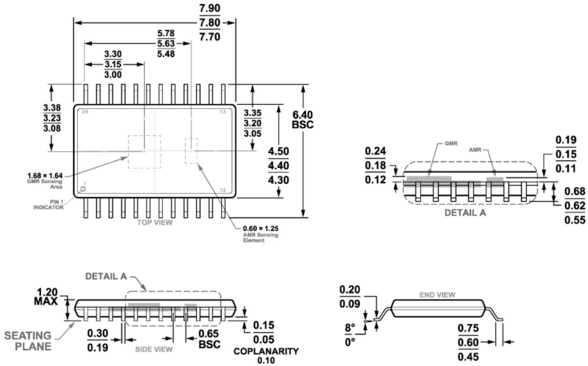
Figure 30. 24-Lead Thin Shrink Small-Outline Package [TSSOP] (RU-24)
