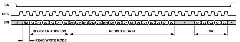
Figure 19. 32-Bit Write Operation for 16-Bit Register
