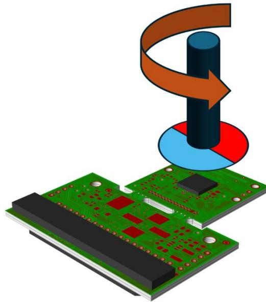
**Figure 20. EV-ADMT4000SDV Evaluation Board in an End-of-Shaft Configuration**
