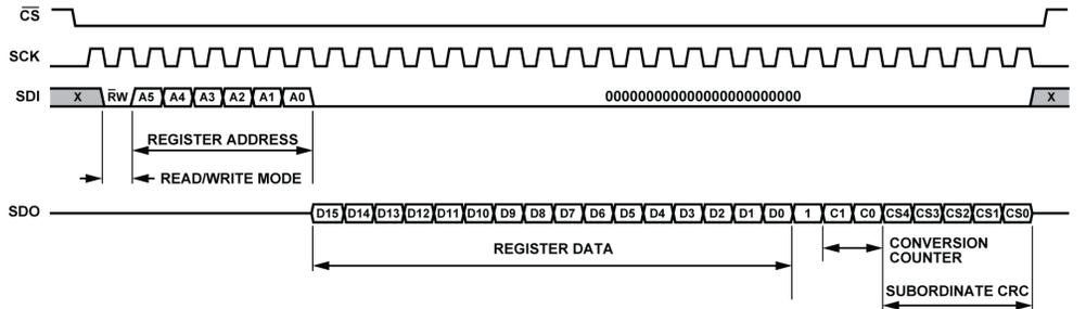
Figure 18. SPI Register Read Operation
