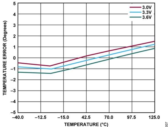
Figure 7. Temperature Sensor Error vs. Ambient Temperature
