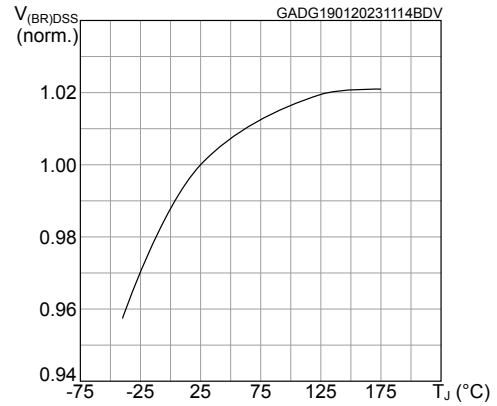
Figure 8. Normalized breakdown voltage vs temperature
