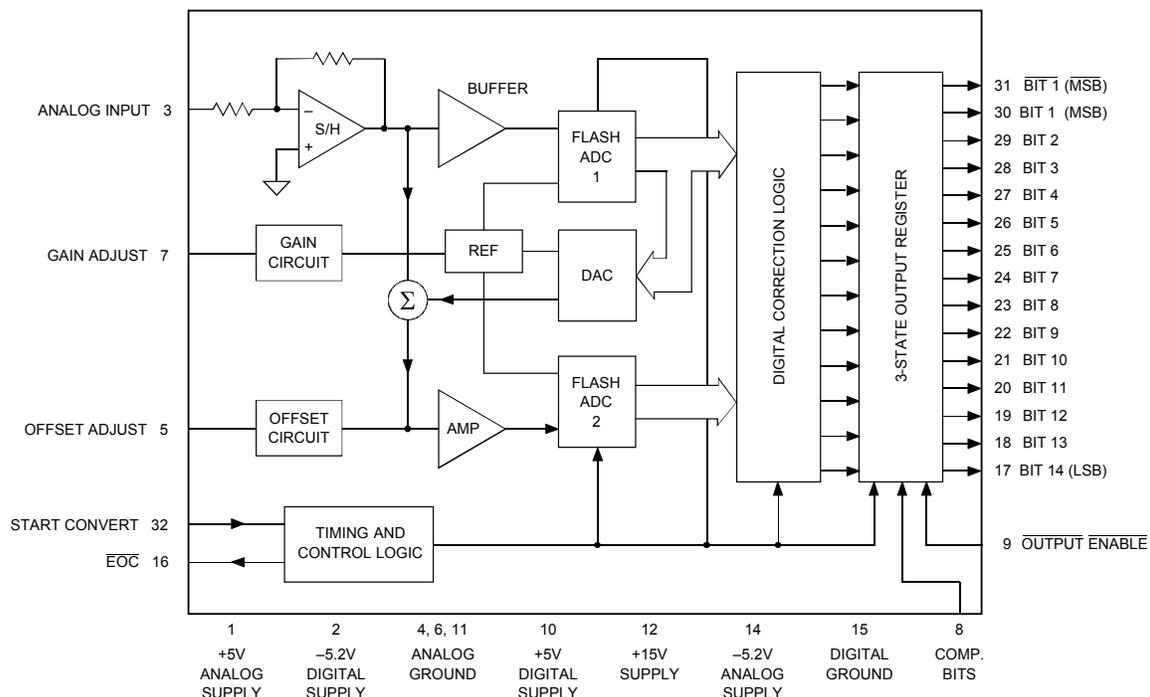
Figure 1. ADS-944 Functional Block Diagram
