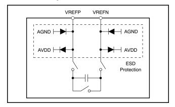
Figure 67. Equivalent Reference Input Circuitry
