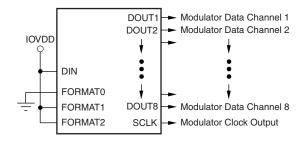
Figure 82. Modulator Output
