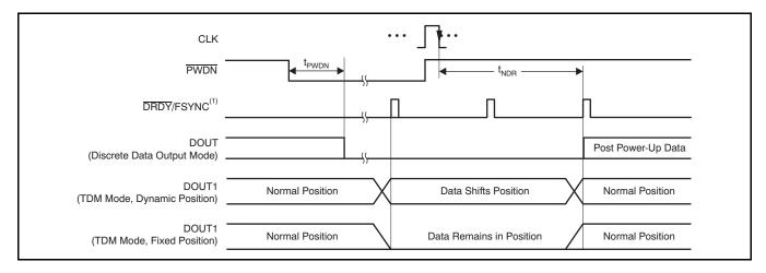
Figure 72. Power-Down Timing
