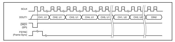
Figure 79. Daisy-Chain Data Format of Figure 78
