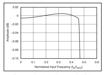
Figure 60. Passband Response for High-Resolution Mode
