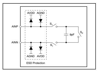
Figure 64. Equivalent Analog Input Circuitry
