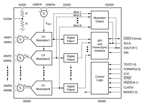
Figure 54. Block Diagram
