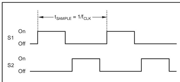
**Figure 40. Timing for the Switches in Figure 39**
