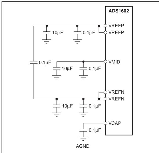
Figure 43. Reference Bypassing When Using the Internal Reference
