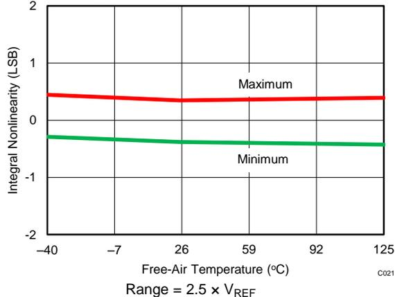
Figure 21. INL vs Temperature ( $2.5 \times V_{REF}$ )
