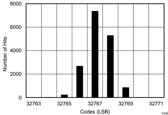
**Figure 65. DC Histogram for Mid-Scale Input (AUX Channel)**
