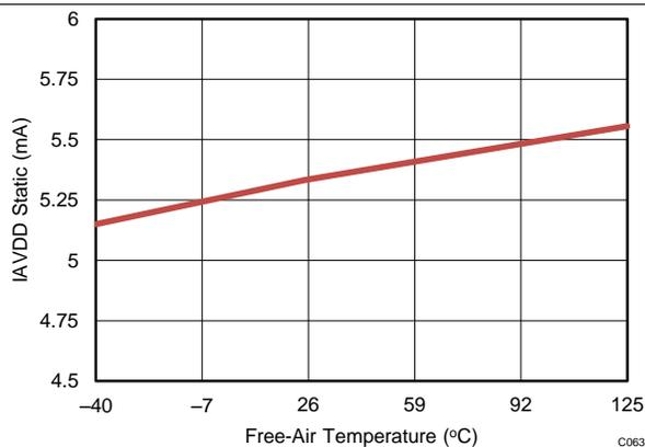
Figure 48. AVDD Current vs Temperature for the ADS8684 (During Sampling)
