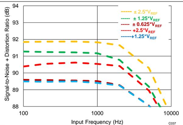
Figure 37. SINAD vs Input Frequency
