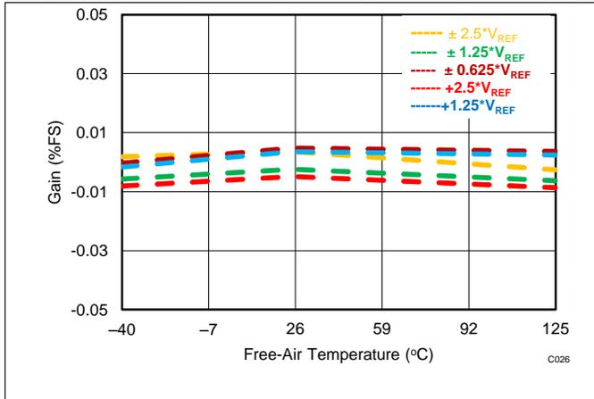
Figure 26. Gain Error vs Temperature Across Input Ranges
