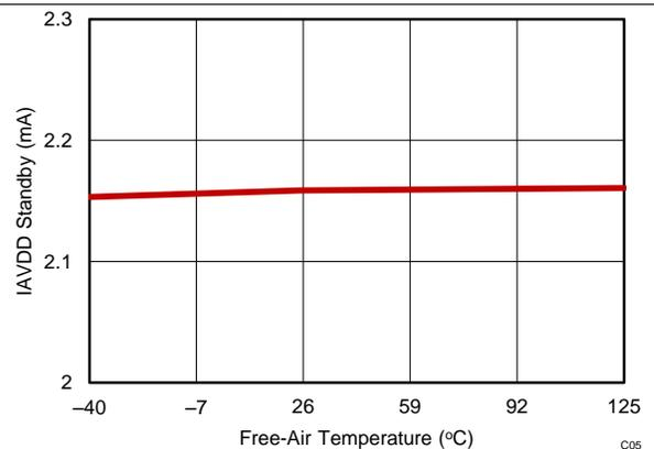
Figure 49. AVDD Current vs Temperature (STANDBY)
