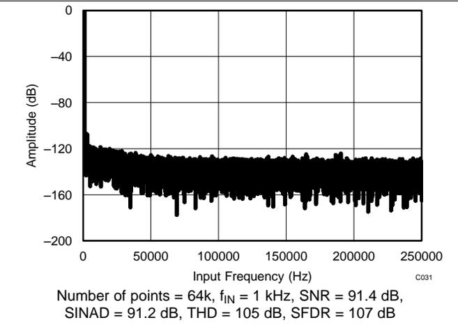
Figure 31. Typical FFT Plot ( $\pm 1.25 \times V_{REF}$ )
