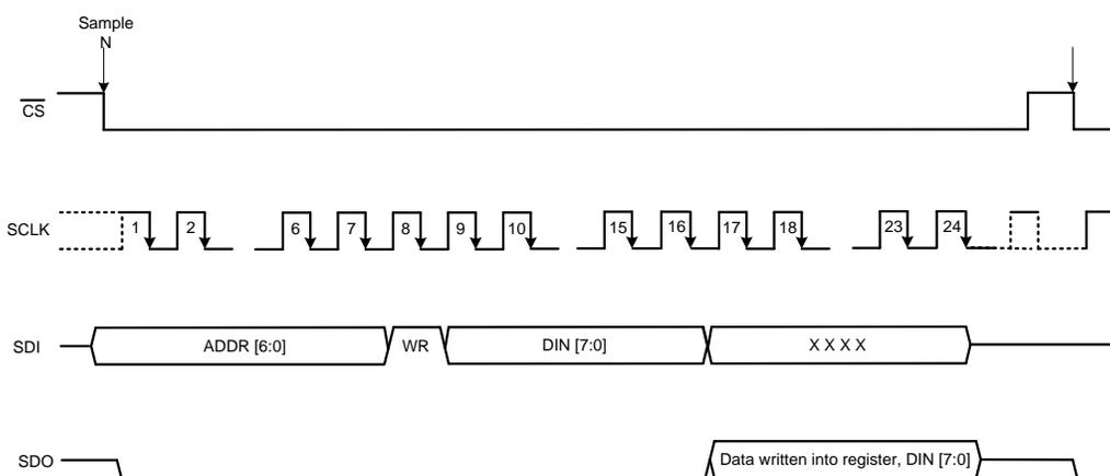
**Figure 88. Program Register Write Cycle Timing Diagram**
