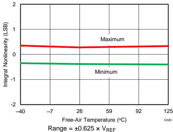
Figure 20. INL vs Temperature ( $\pm 0.625 \times V_{REF}$ )
