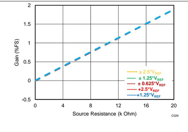
Figure 29. Gain Error vs External Resistance ( $R_{EXT}$ )
