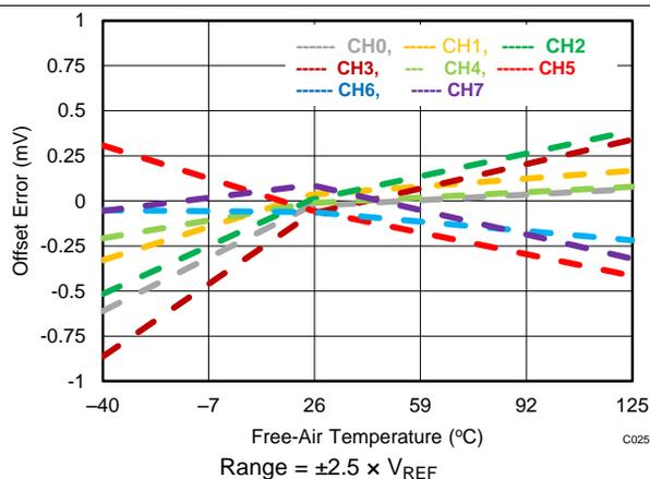
Figure 25. Offset Error vs Temperature Across Channels
