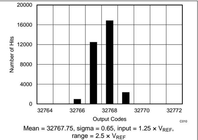
Figure 9. DC Histogram for Mid-Scale Inputs ( $2.5 \times V_{REF}$ )
