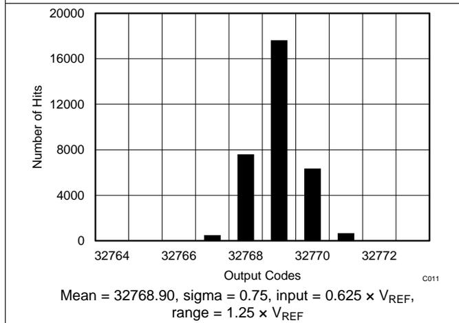
Figure 10. DC Histogram for Mid-Scale Inputs ( $1.25 \times V_{REF}$ )
