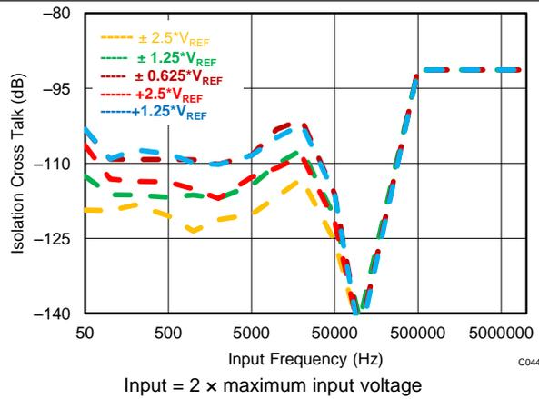
Figure 44. Isolation Crosstalk vs Frequency for Overrange Inputs
