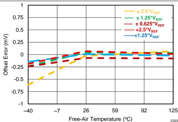
Figure 23. Offset Error vs Temperature Across Input Ranges
