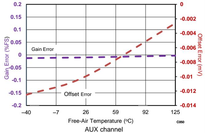
**Figure 66. Offset and Gain vs Temperature (AUX Channel)**
