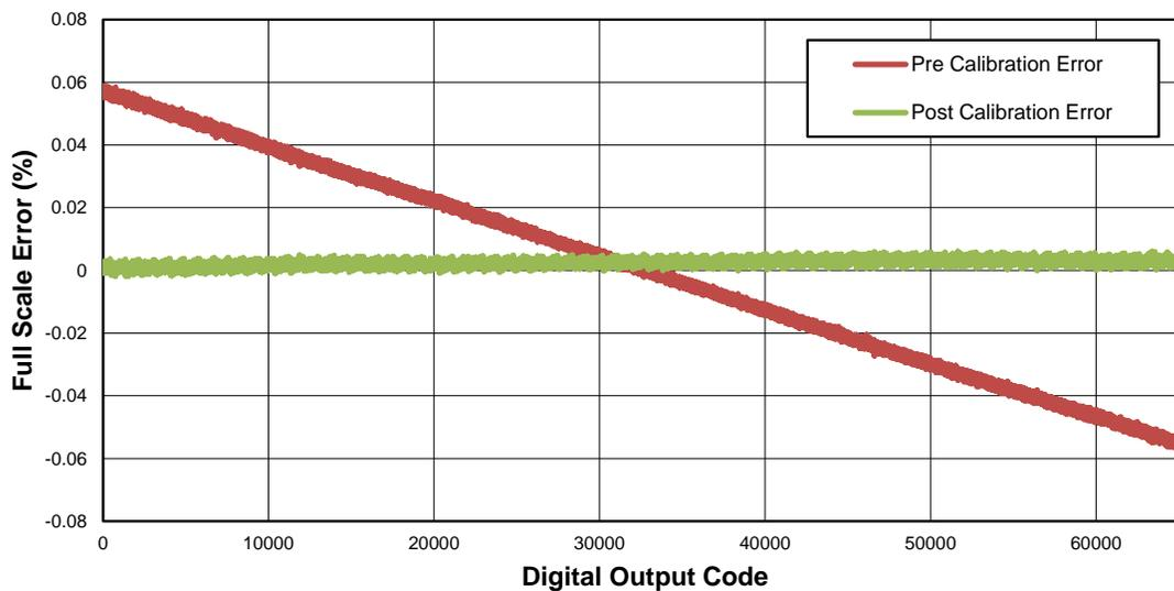
**Figure 98. System Accuracy Performance in ±2.5 × V<sub>REF</sub> Input Range**
