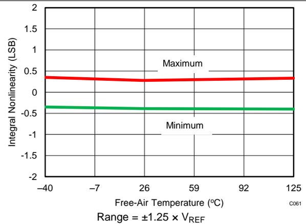
Figure 19. INL vs Temperature ( $\pm 1.25 \times V_{REF}$ )
