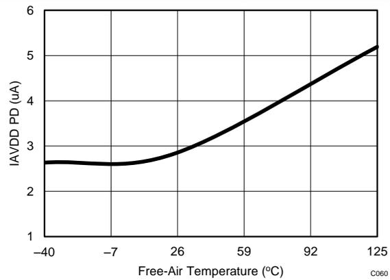
**Figure 50. AVDD Current vs Temperature
