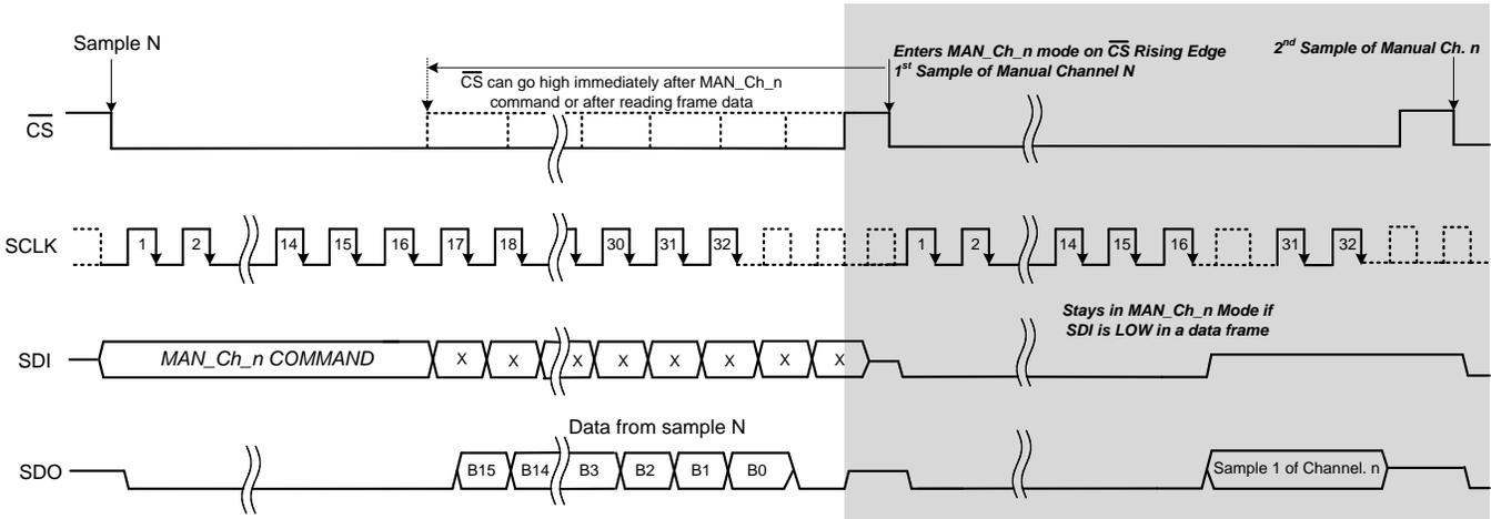
Figure 83. Enter MAN\_Ch\_n Scan Mode Timing Diagram
