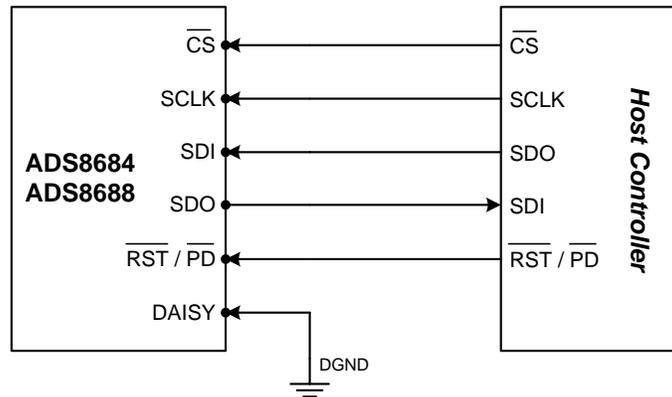
**Figure 70. Pin Configuration for the Digital Interface**
