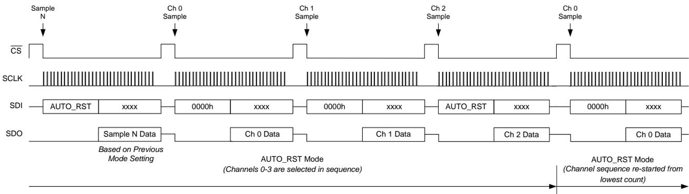
Figure 82. Device Operation Example in AUTO\_RST Mode
