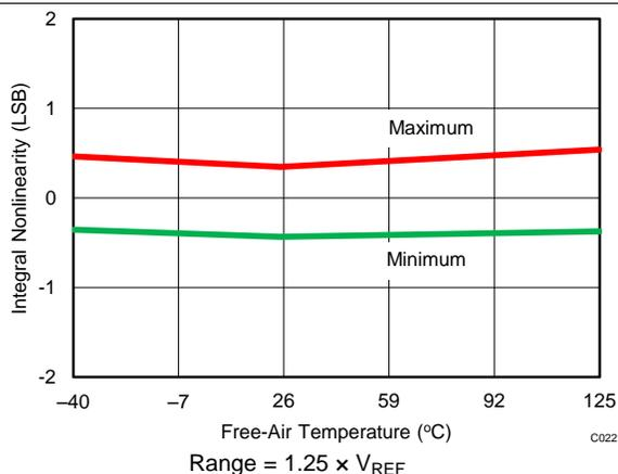
Figure 22. INL vs Temperature ( $1.25 \times V_{REF}$ )
