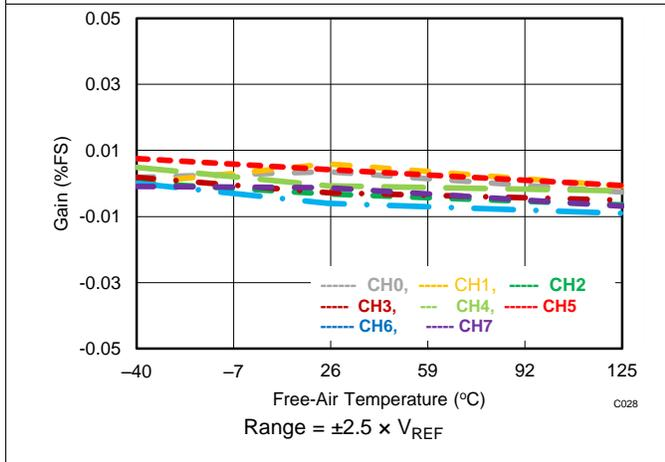
Figure 28. Gain Error vs Temperature Across Channels
