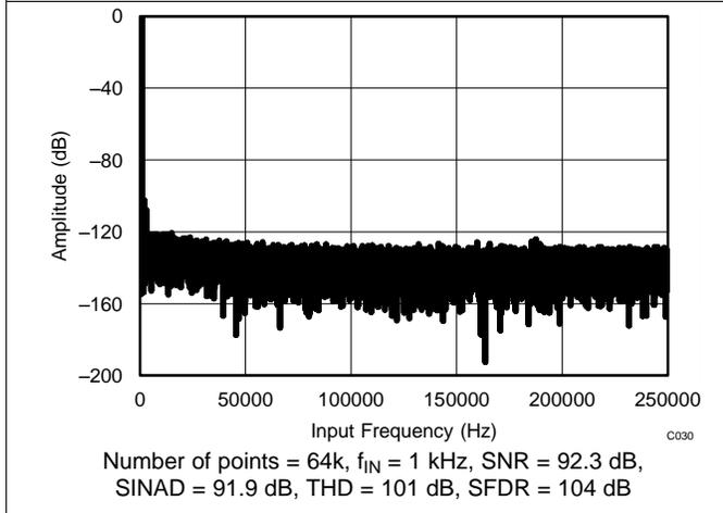
Figure 30. Typical FFT Plot ( $\pm 2.5 \times V_{REF}$ )
