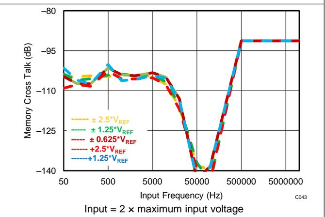
Figure 43. Memory Crosstalk vs Frequency for Overrange Inputs
