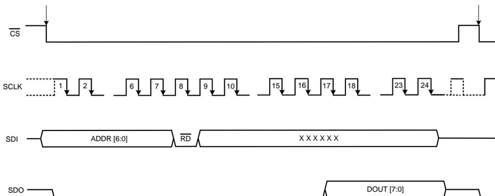
**Figure 89. Program Register Read Cycle Timing Diagram**
