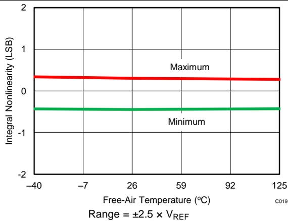
Figure 18. INL vs Temperature ( $\pm 2.5 \times V_{REF}$ )
