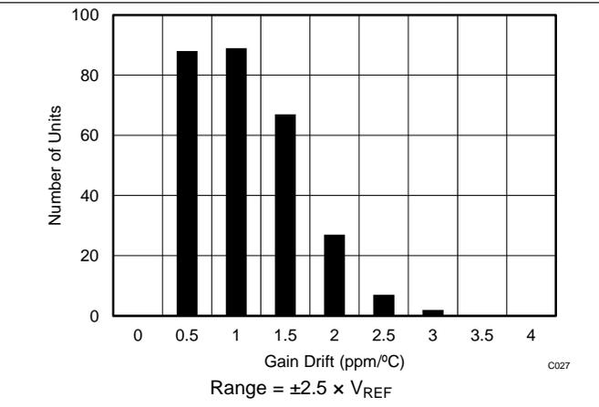
Figure 27. Typical Histogram for Gain Error Drift
