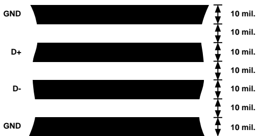
Figure 12. Arrangement of Signal Tracks
