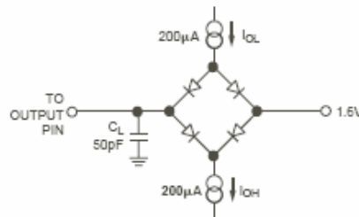
Figure 2. Load Circuit for Access Time and Bus Relinquish Time
