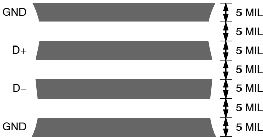
Figure 16. Typical Arrangement of Signal Tracks
