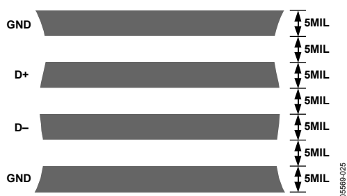
Figure 35. Typical Arrangement of Signal Tracks
