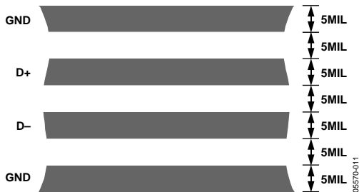
Figure 22. Typical Arrangement of Signal Tracks
