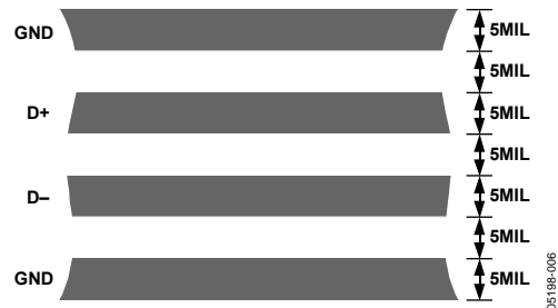
Figure 18. Arrangements of Signal Tracks
