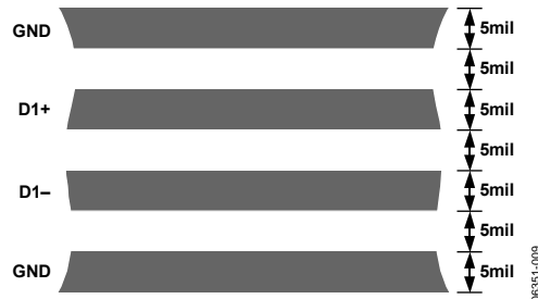
Figure 18. Arrangements of Signal Tracks
