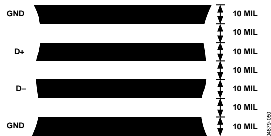
Figure 50. Arrangement of Signal Tracks
