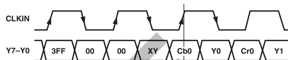
Figure 18a. Cb Data on Rising Edge—Clock Edge Address 01h Bit 1 Should be Set to 0
