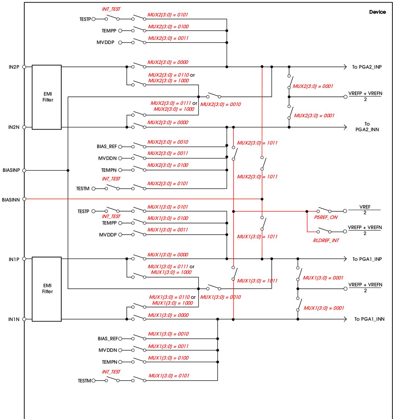
NOTE: MVDD monitor voltage supply depends on channel number; see the Supply Measurements (MVDDP, MVDDN) section.
