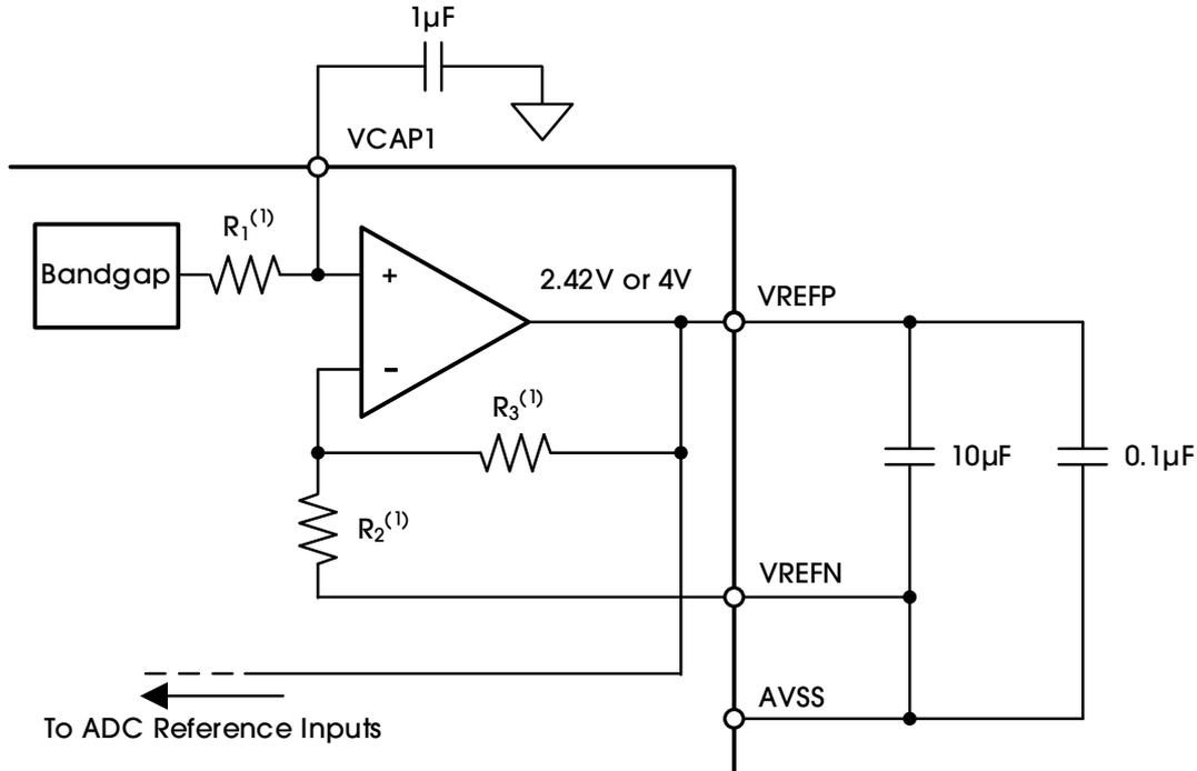
(1) For  $V_{REF} = 2.42V$ :  $R_1 = 100k\Omega$ ,  $R_2 = 200k\Omega$ , and  $R_3 = 200k\Omega$ . For  $V_{REF} = 4V$ :  $R_1 = 84k\Omega$ ,  $R_2 = 120k\Omega$ , and  $R_3 = 280k\Omega$ .
