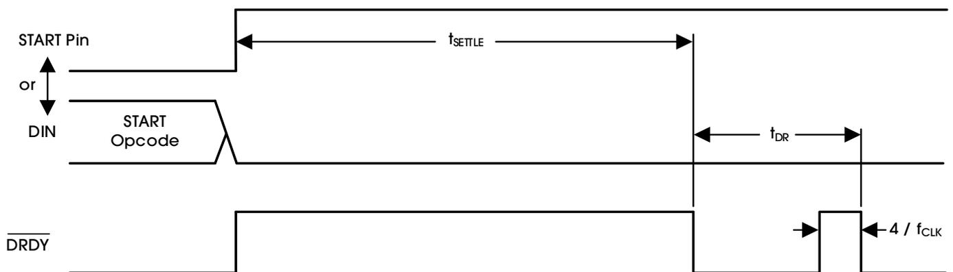
(1) Settling time uncertainty is one  $t_{\text{MOD}}$  cycle.
