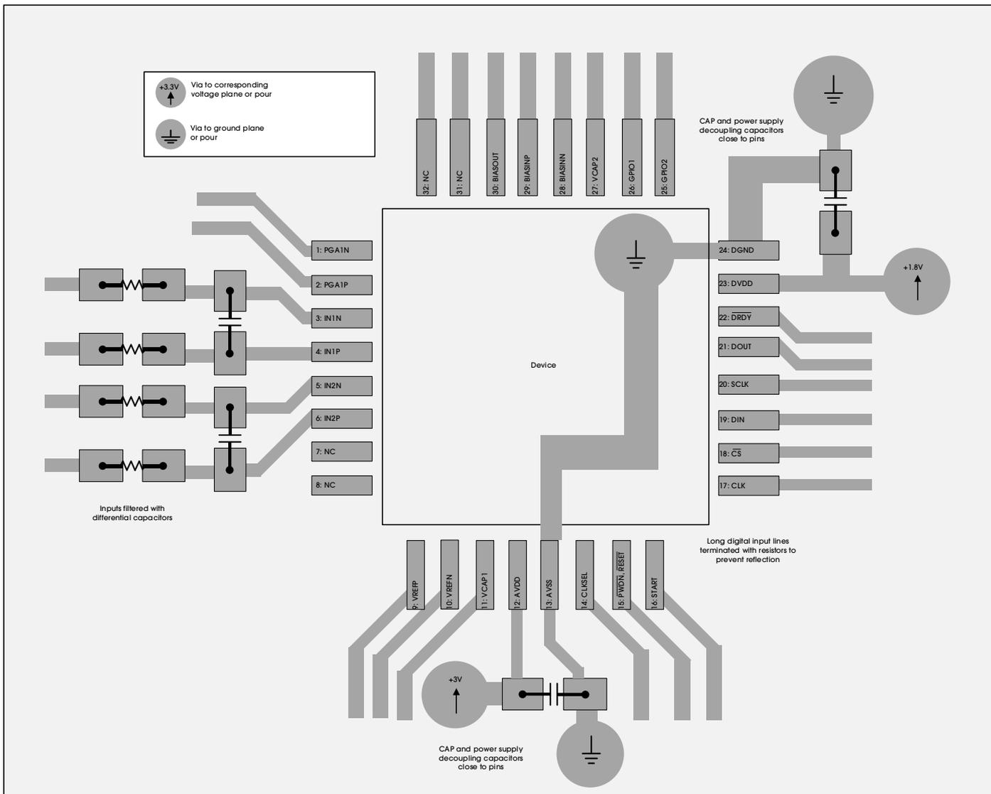
Figure 62. Example PCB Layout for Single-Supply Operation
