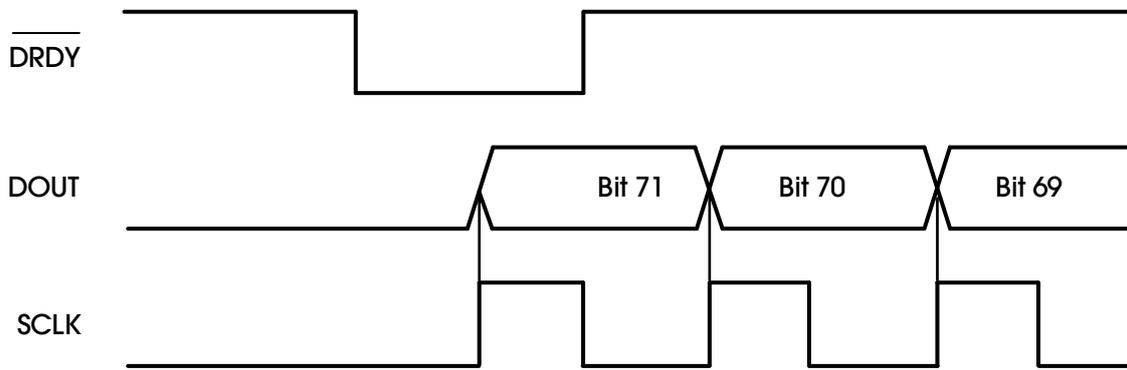
Figure 48.  $\overline{\text{DRDY}}$  with Data Retrieval ( $\overline{\text{CS}} = 0$ )
