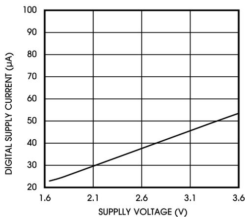
Figure 14. Digital Supply Current vs. Supply Voltage
