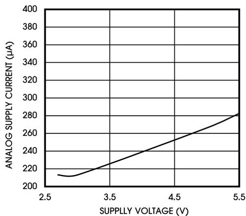
Figure 12. Analog Supply Current vs. Supply Voltage
