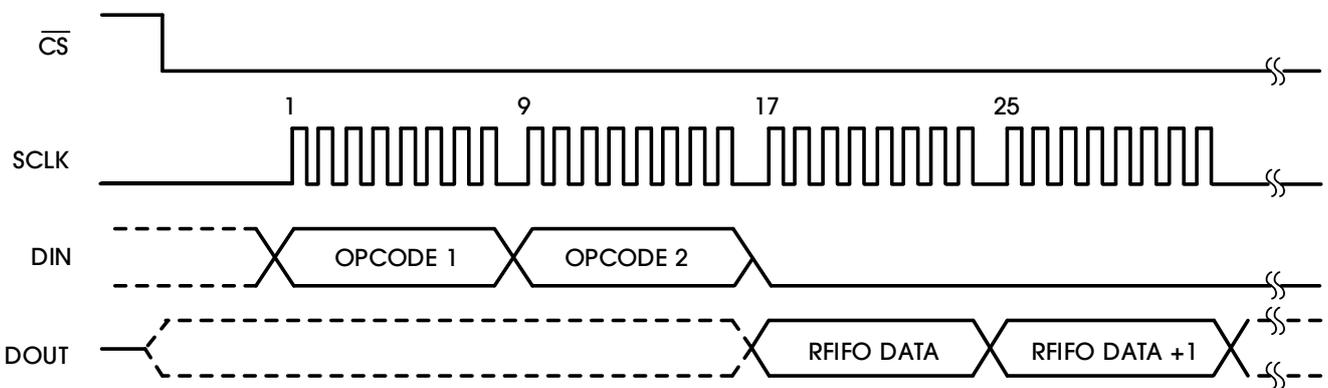
Figure 57. RFIFO Command Example: Read Two Registers Starting from FIFO
