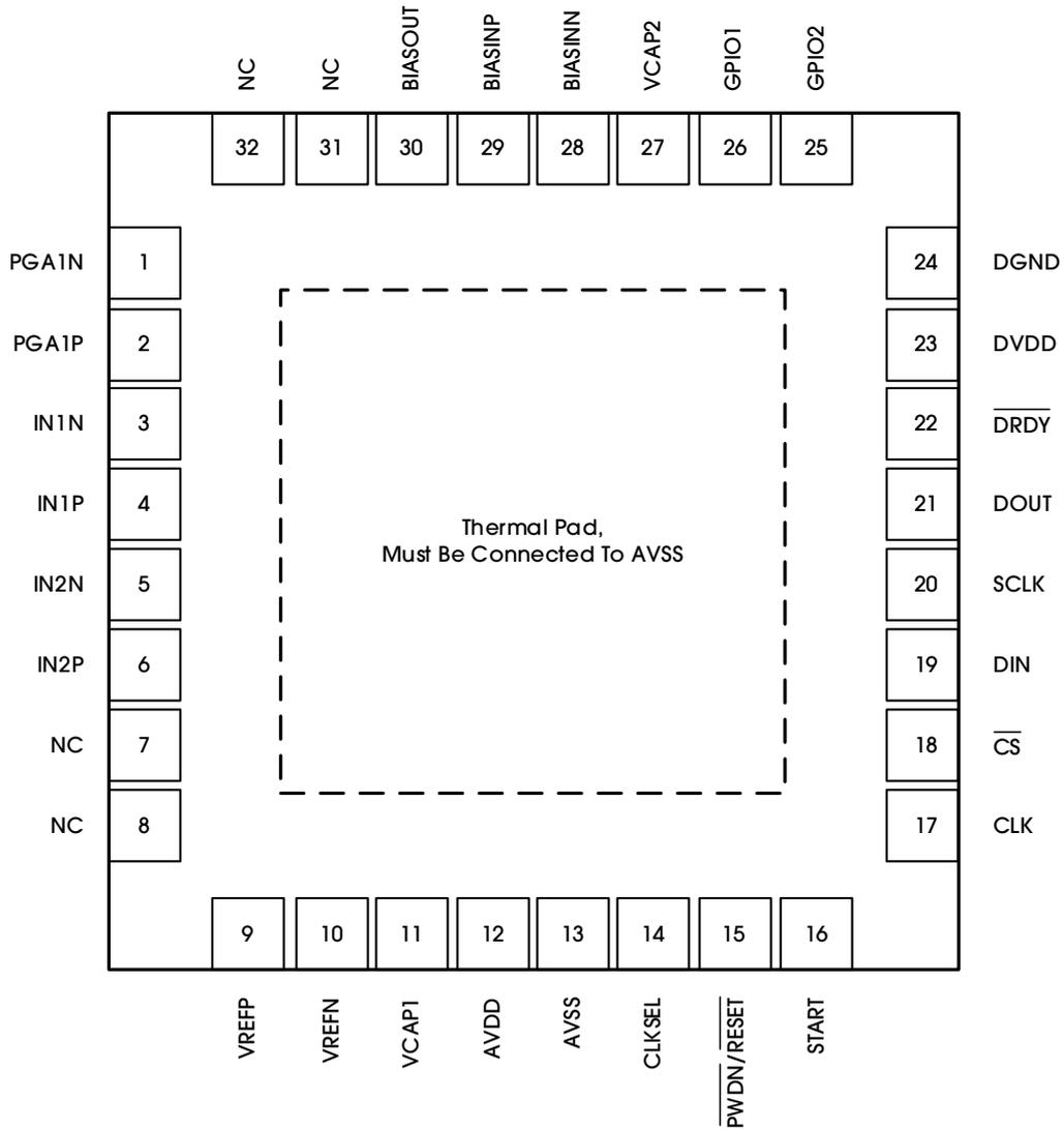
Figure 2. Pin Configuration (ADX3202Q)
