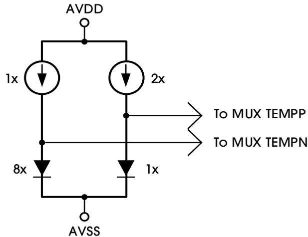
Figure 21. Temperature Sensor Measurement in the Input
