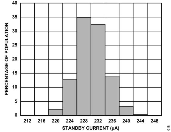
Figure 19. ADXL1001/ADXL1002 Standby Current Histogram at 5 V
