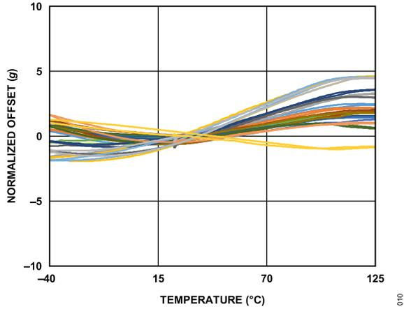
Figure 10. ADXL1001 Normalized Offset vs. temperature
