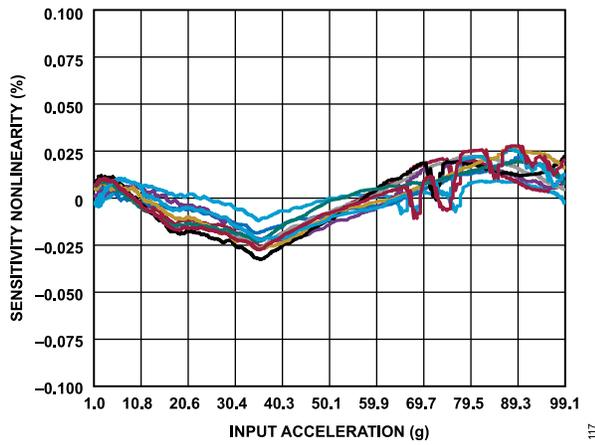
Figure 17. ADXL1001 Sensitivity Nonlinearity vs. Input Acceleration
