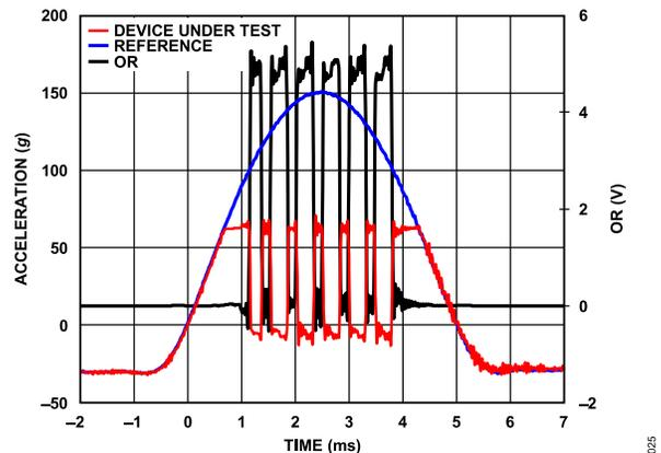
Figure 26. ADXL1001/ADXL1002 Behavior During a Continuous Overrange
