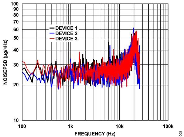
Figure 8. ADXL1002 Noise Power Spectral Density (PSD)
