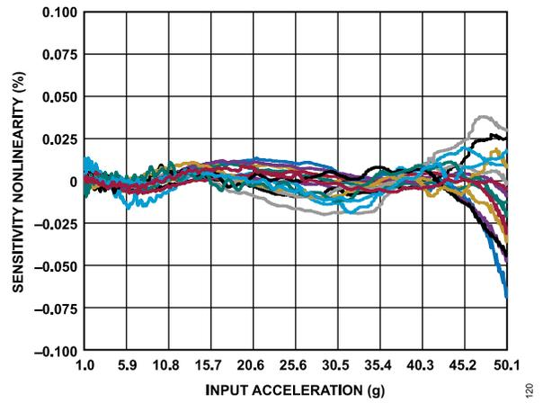
Figure 20. ADXL1002 Sensitivity Nonlinearity vs. Input Acceleration
