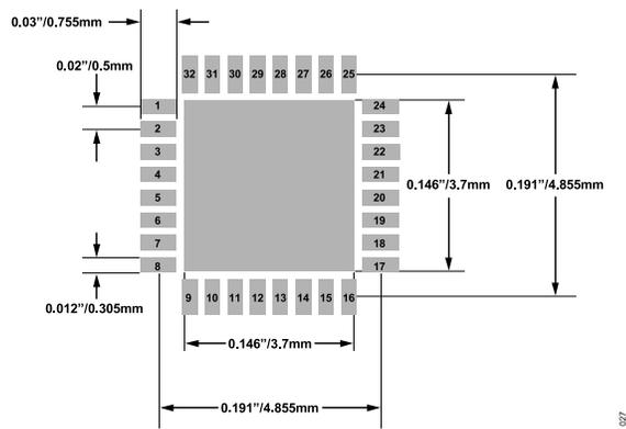
Figure 28. Recommended Printed Wiring Board Land Pattern
