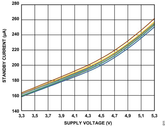
Figure 11. ADXL1001/ADXL1002 Standby Current vs. Supply Voltage
