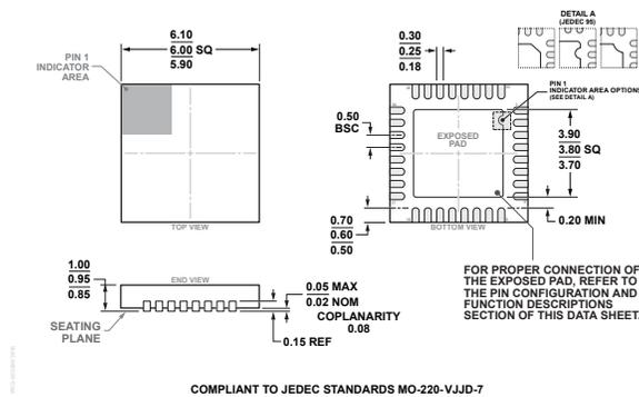
**Figure 4. 32-Lead Lead Frame Chip Scale Package [LFCSP]
