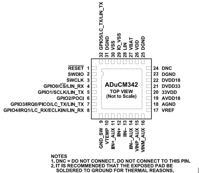
Figure 2. Pin Configuration
