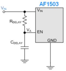
For example, setting V<sub>IN</sub>=24V, R<sub>DELAY</sub>=100K $\Omega$ , C<sub>DELAY</sub> =0.1uF. The start-up delay time can be calculated as below:
