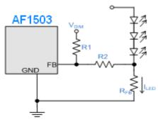
If the  $V_{\text{DIM}}$  is taken below the VFB, the inverse will happen and brightness will increase.
