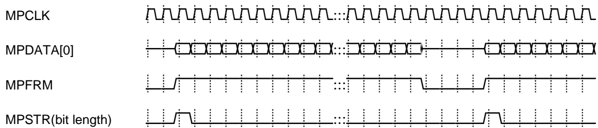
Figure 13: Timing diagram of the AF9015 MPEG-2 TS serial input interface.
