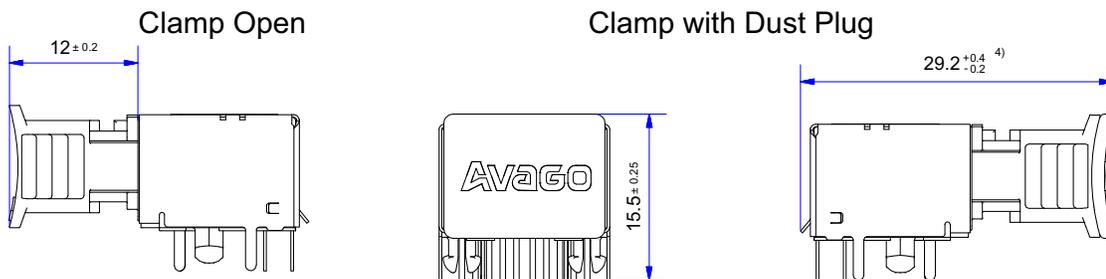
**Figure 5: AFBR-59F2Z Transceiver Module with Dust Plug**
