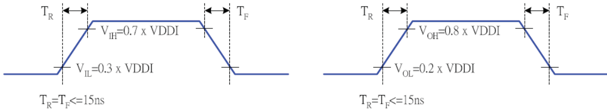
Fig. 8.1.2 Rising and falling timing for input and output signal
