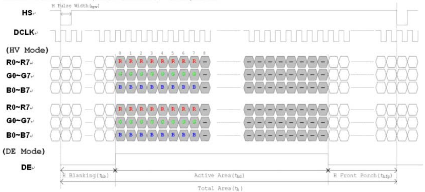
Horizontal input timing diagram.
