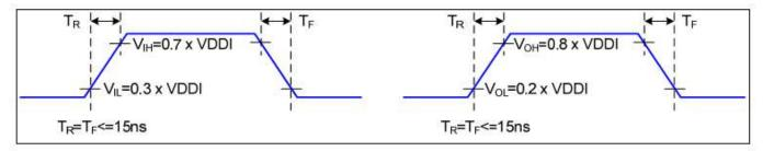
Figure 2 Rising and Falling Timing for I/O Signal
