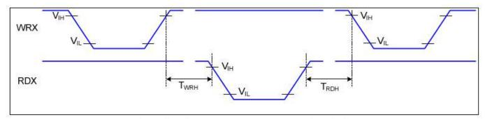
Figure 3 Write-to-Read and Read-to-Write Timing
