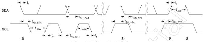
Figure 7 I2C Fast Mode Timing
