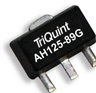
3-pin SOT-89 Package
