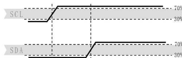
Figure 19. Stop transmission state (P)
