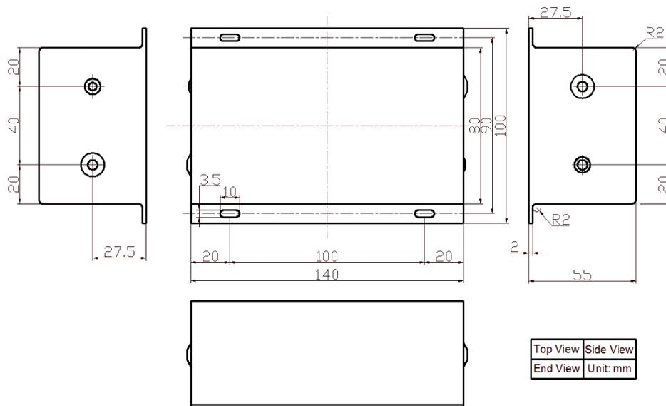
Figure 12. Dimensions for AHV24V25KV1MAW
