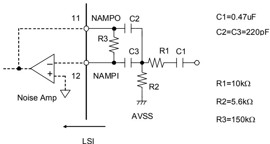
$$(1) \quad f_0 = \frac{1}{2\pi\sqrt{R_3(R_1//R_2)C^2}}$$
