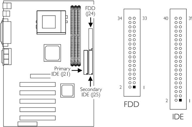
If you encountered problems while using an ATAPI CD-ROM drive that is set in Master mode, please set the CD-ROM drive to Slave mode. Some ATAPI CD-ROMs may not be recognized and cannot be used if incorrectly set in Master mode.
