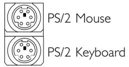
Make sure to turn off your computer prior to connecting or disconnecting a mouse or keyboard. Failure to do so may damage the system board.
