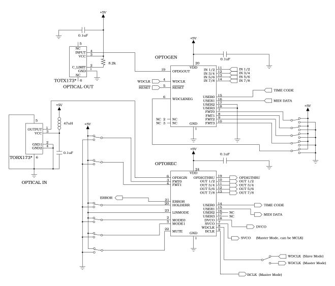
\* Optical I/O parts shown are Toshiba parts. The Sharp GP1F33RT or equivalent is also compatible.
