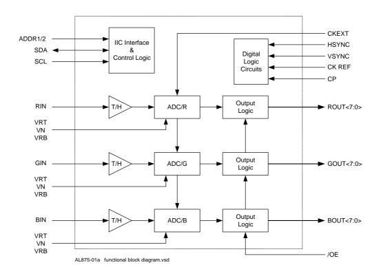
The AL875 is a high-speed triple 8-bit monolithic analog-to-digital converter (ADC) designed for digitizing RGB graphics/video signal or other applications. Its 110 MHz conversion rate can support display resolution of up to 1280x1024 at 60Hz refresh rate.
