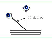
Under daylight lamp 20 ${\sim}40W_{\textrm{F}}\,$  product distance inspector 'eye 30cm,incline degree 30°.
