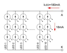
The constant current source is needed for white LED back-light driving. back-light should be adjusted to 135mA max
