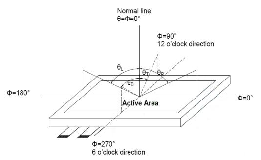
Note 2: Definition of optical measurement system.
