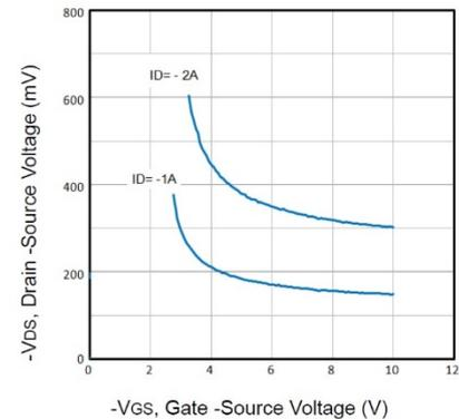
Fig5. Typical Source-Drain Diode Forward Voltage
